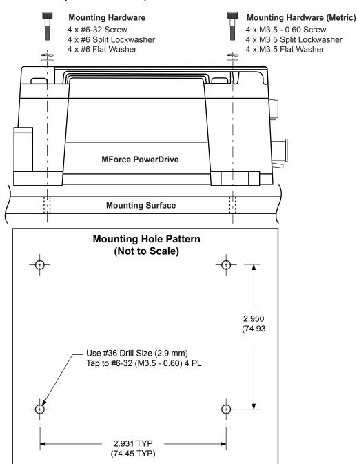
Figure 2.1.1: Base Mounting the MForce PowerDrive
